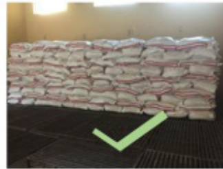
Stacking of HDPE bags by Brick layer method
